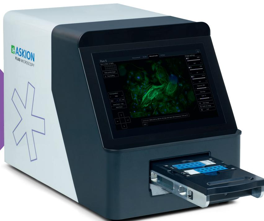
**FluoS** is an intuitive platform for entry-level fluorescence microscopy. Designed as a stand-alone system, it features an intuitive touchscreen interface that simplifies navigation and operation—even for inexperienced users.
